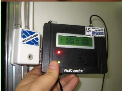
The sensors are to be installed on the distance up to 5 m from each other and from the data transmission unit. The transmission unit includes a common SIM card for mobile data forwarding to central unit/owner's mobile phone/analytical center ViziCounterOnline. The control unit provides the button allowing to switch the counter into protection mode when each crossing in the undue time is reported to owner via SMS.
