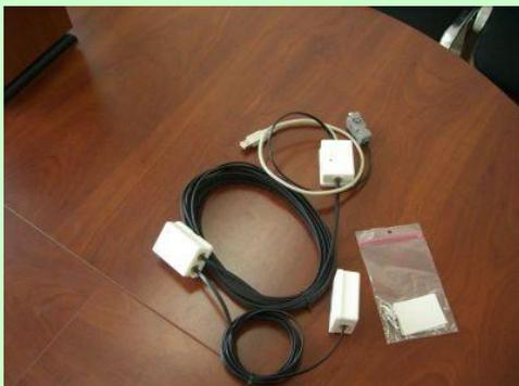
The sensors are to be installed on the distance up to 5 m from each other. They are logging all the crossings of the line between them. Features:
